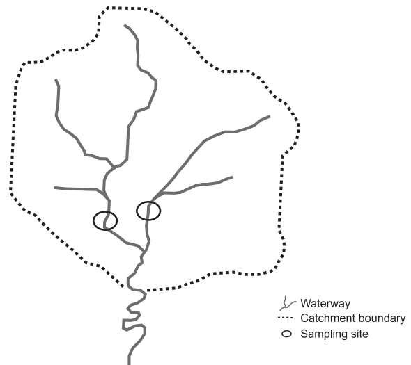
Figure 4–3 Model of monitoring site placement when comparing subcatchments (modified from Cassidy 2003)
